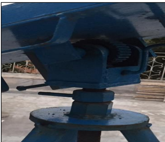
Fig 1: Power Screw for Altering Line
